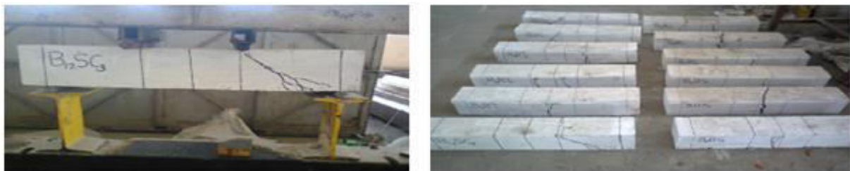
Fig. 3- Shear failure of beam with mild steel as reinforcement and beam after crack
